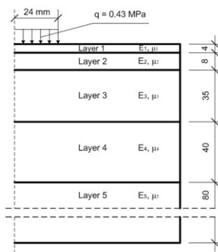
**Fig. 5.** Pavement structure model adopted for the calculations
