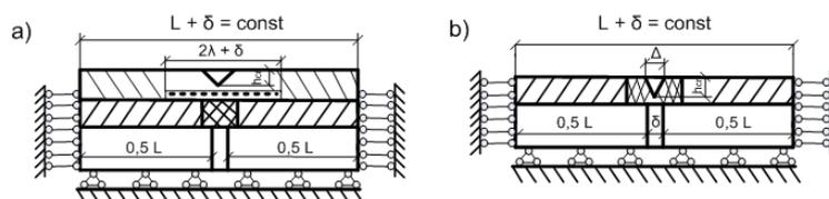
**Fig. 4.** Design models for the calculation of stresses in asphalt concrete pavement after the repair and re-crack formation:
