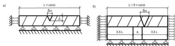
**Fig. 2.** Design models for the calculation of stresses in asphalt concrete pavement after crack appearance:
