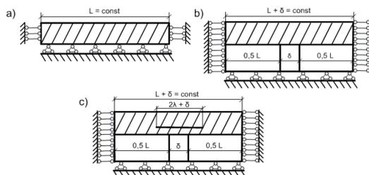
**Fig. 1.** Design models for the calculation of stresses in asphalt concrete pavement before cracking:
