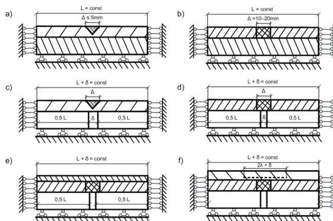
**Fig. 3.** Design models for the calculation of stresses in asphalt concrete pavement after repairing activities:
